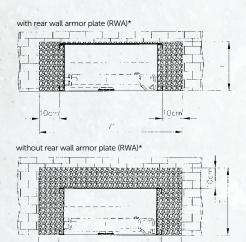
Wall safe should be placed centred. Leave a gap of at least 10 cm to the masonry.
